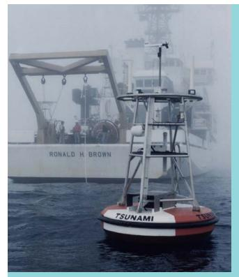
A DART buoy in the northern Pacific, near the Aleutian Islands, receives information from an instrument on the seafloor that calculates wave height. The buoy relays that information to satellites, which bounce it to regional warning centers.
